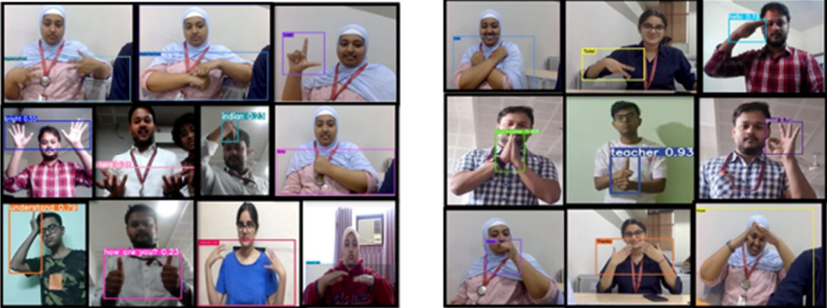
Fig.5 Detection of 20 gestures of the ISL (Indian Sign Language) in real time
