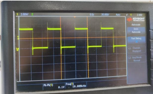
Fig 5.TLP350 Output Designed to Drive Buck converter at 20 kHz sampling frequency
